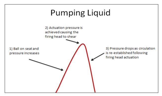
• If the fluid being used to pump a ball down-hole is a liquid followed by nitrogen the expected pressure profile should be similar to the diagram below.
