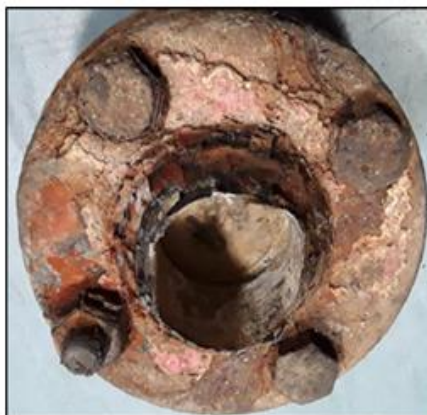
Figure 2. Deluge Line Blanking Plate
