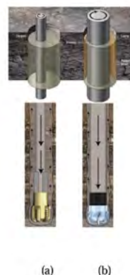
Fig. 9. (a) Conventional drilling, and (b) CwD wellbore geometry
