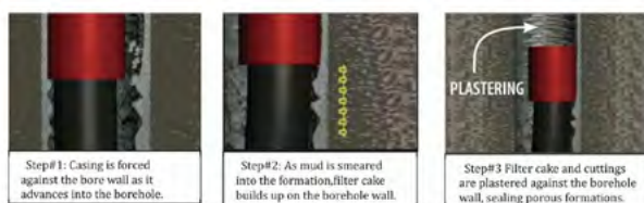
Fig. 7. Plastering effect in the casing while drilling operation.
