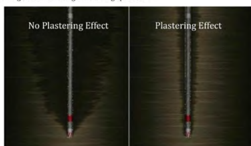
Fig. 8. Illustration of plastering effect.
