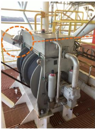
Figure 1 - VIKING Norsafe davit winches NW-150-NO
