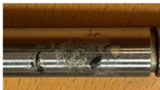
Disassembly of the lifeboat davit gas strut showing corrosion
