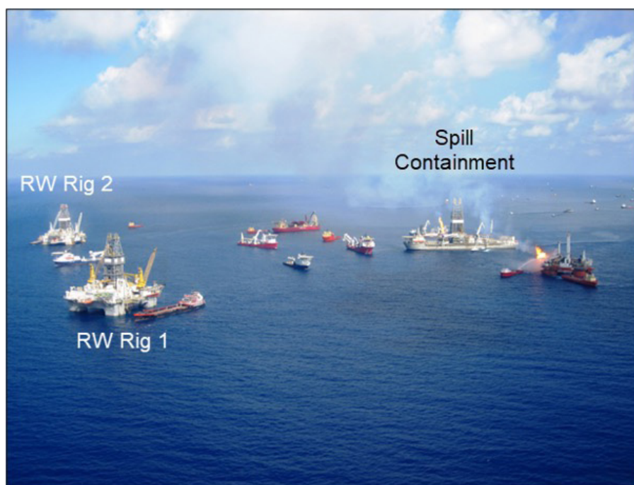
Figure 4 – Example of multi-vessel SIMOPS during blowout containment and relief well operation in deepwater (relief well rigs are in this case ~850 m from spill site).
