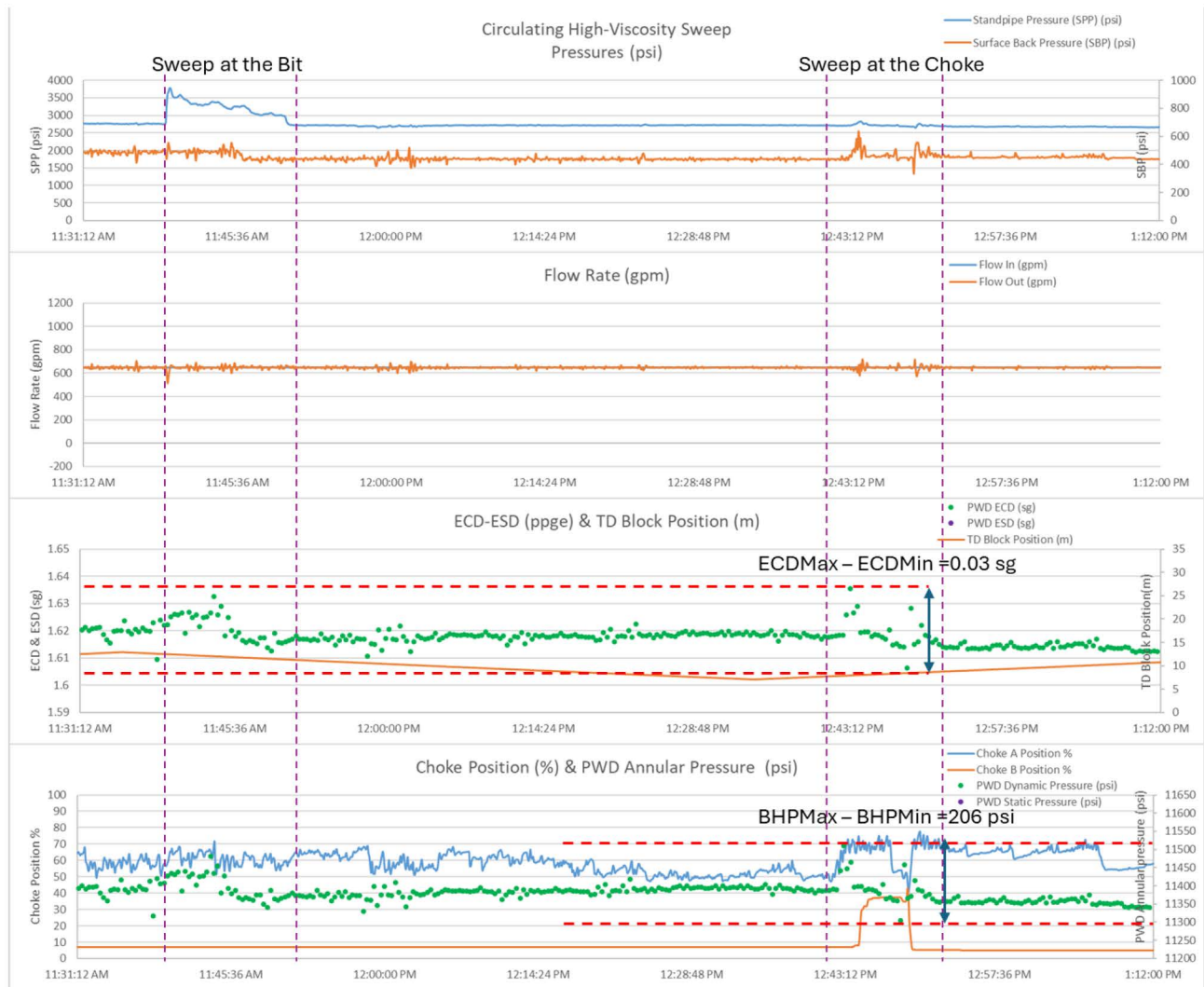
Figure 4—Choke Behavior and BHP while circulating a 25 bbl Hi-Vis Sweep
