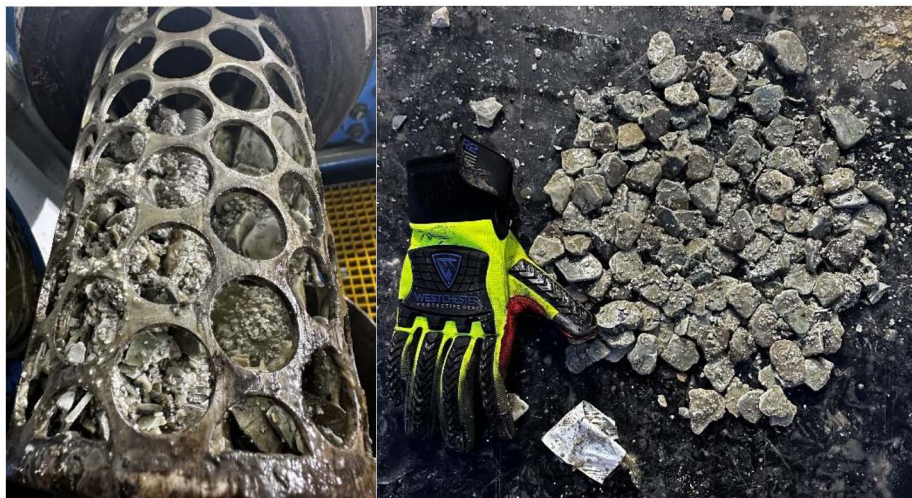
Figure 6—Full Strainer and Cavings captured by the strainers while reaming to well bottom.
