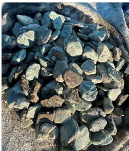
Figure 5—0.75-1.25" Cavings removed from the strainers after stuck pipe event
