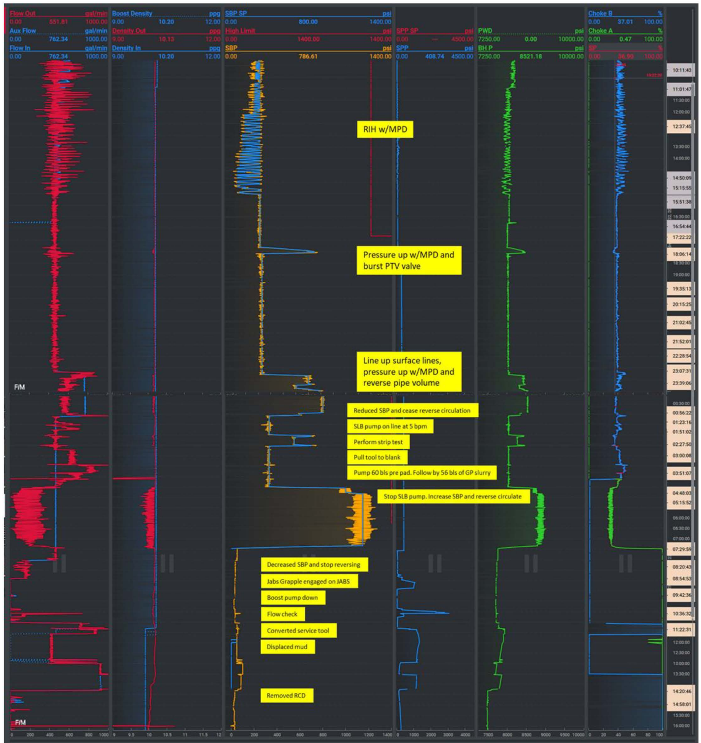
Figure 6—MPD system user interface time-based plots – Screens RIH and OHGP Well-X
