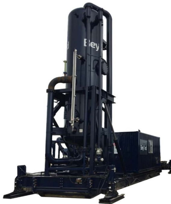
Figure 10—Beyond Mus Gas Separator (Big-B) with Manifold Building behind
