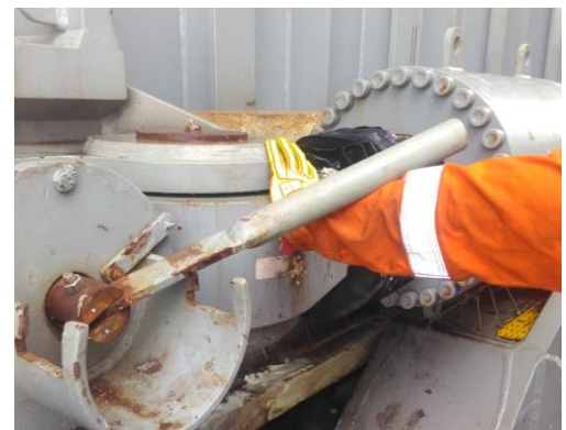
Figure 2: Operating handle struck-by risk
