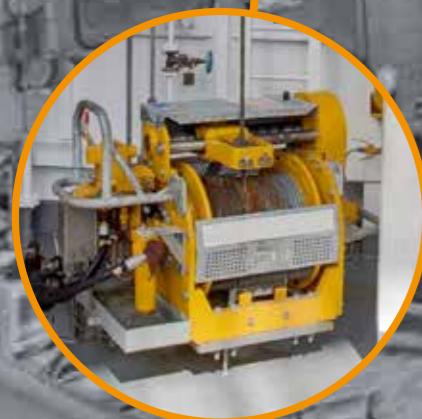
1. Tugger Load Monitoring optimizes general lifting operations on the drill floor
