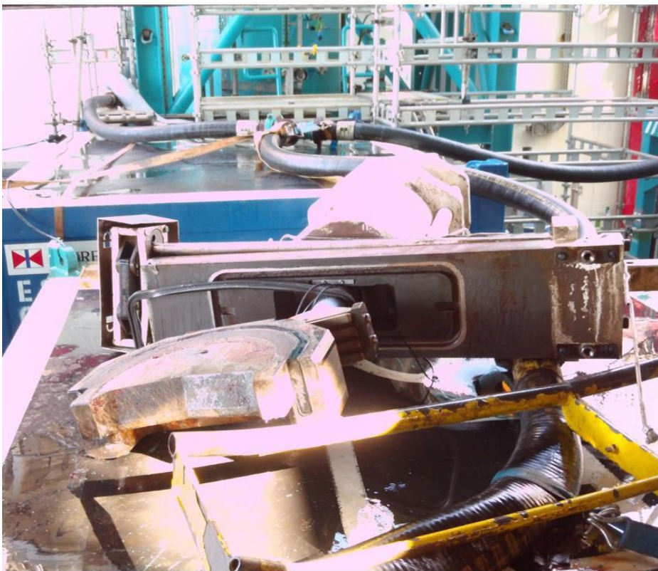
Picture 1: BOP Door and Ram on Top of Container
