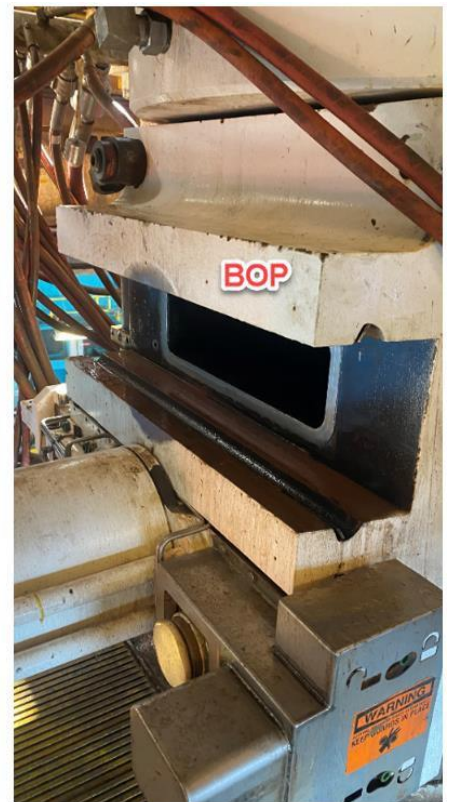
Picture 2: BOP Body Where Door Separated
