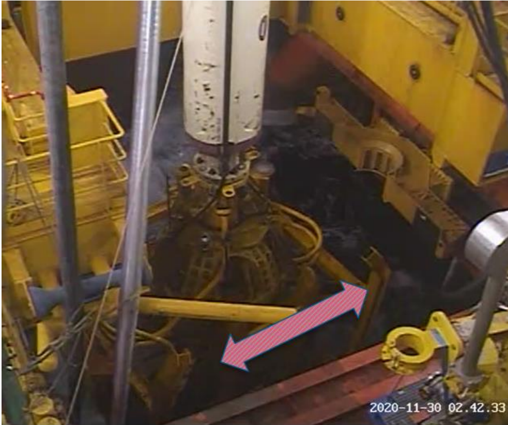
Fig-1: Screenshot from CCTV. Prior to gooseneck ring drop. The riser and BOP can be seen swinging from side to side when BOP is in the splash zone
