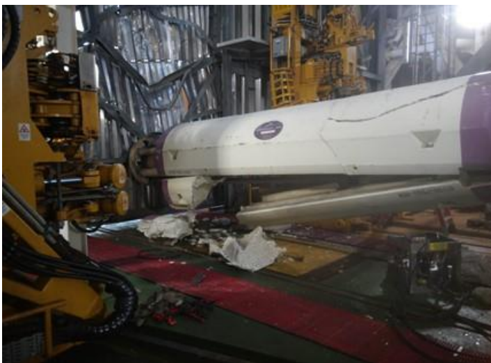
Figure 3 The dropped marine riser hitting the V-door
