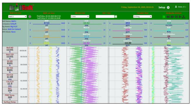
Web Monitoring system streams data through DrillSoft® Real-Time to our servers. Internet connection at the site where Real-Time is necessary to stream data. The Web Monitoring can be accessed anywhere, anytime using your laptop or cell phone. Each client is provided with secure credentials to be able to view the wells. The data on Web Monitoring can be streamed horizontaly or vertically similar to a drilling log.
