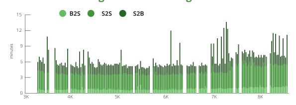
The high level of system utilization produced fast and highly consistent weight to weight times throughout all sections of the well.
