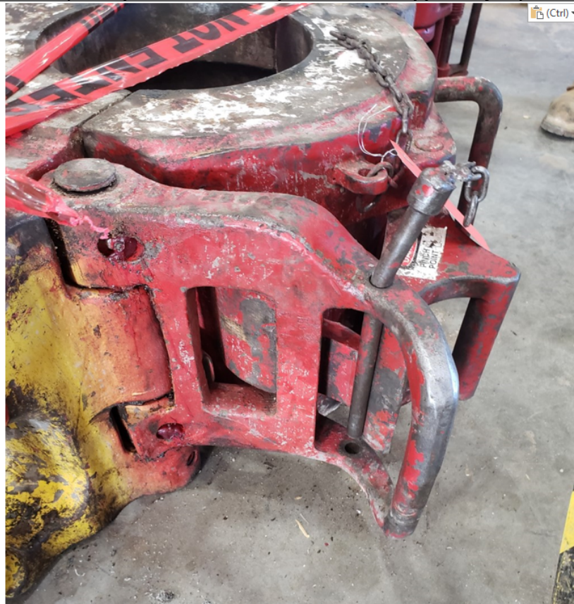
Incorrect pin placement (note: pin was not bent prior to the dropped object)
