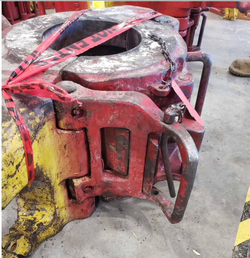
Correct pin placement (note: pin was not bent prior to the dropped object)
