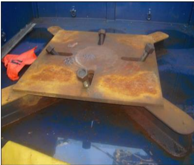
Securing plate BOP was landed on
