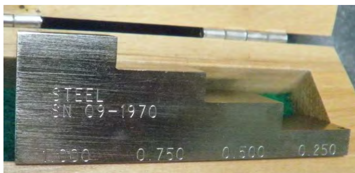
Figure 12: UT Meter Calibration Block
