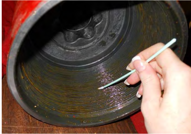
Collecting Grease from Box
