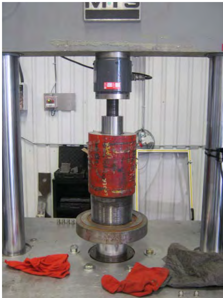
Figure 3.16: Photograph of Flapper Assembly Shear Test
