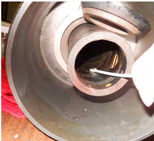
Collecting Residue from Inner Tube
