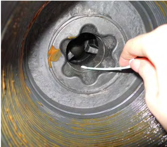
Collecting Residue from Cage Opening
