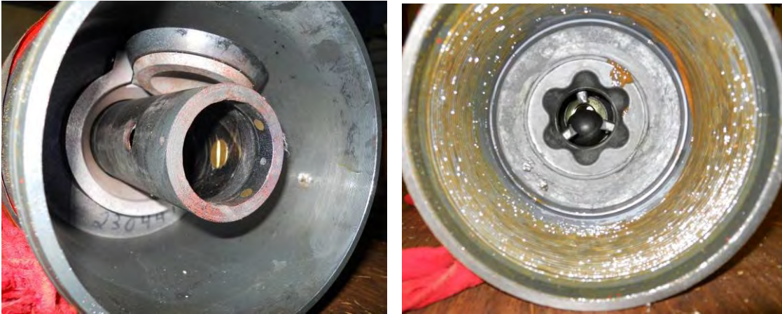
Figure 5: Flapper and Ball Position as-received Sample 1
