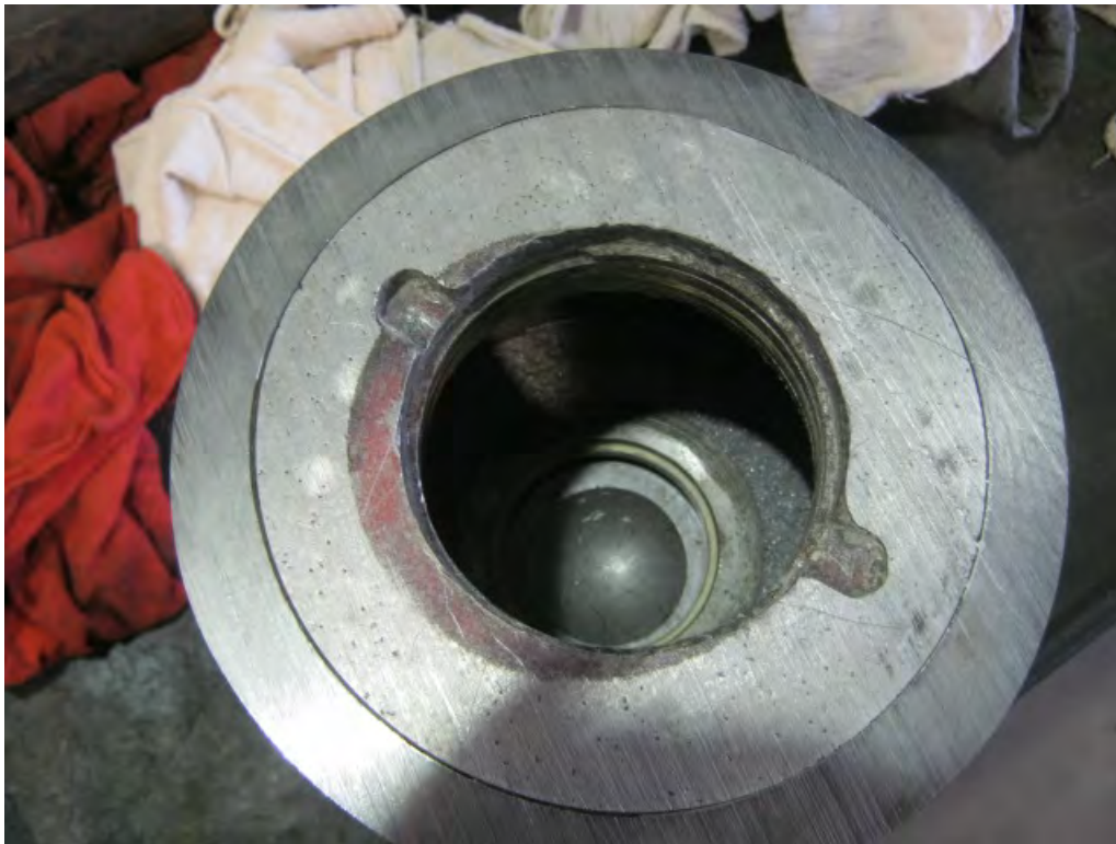
Figure 3.18: Photograph of Flapper Assembly Failure
