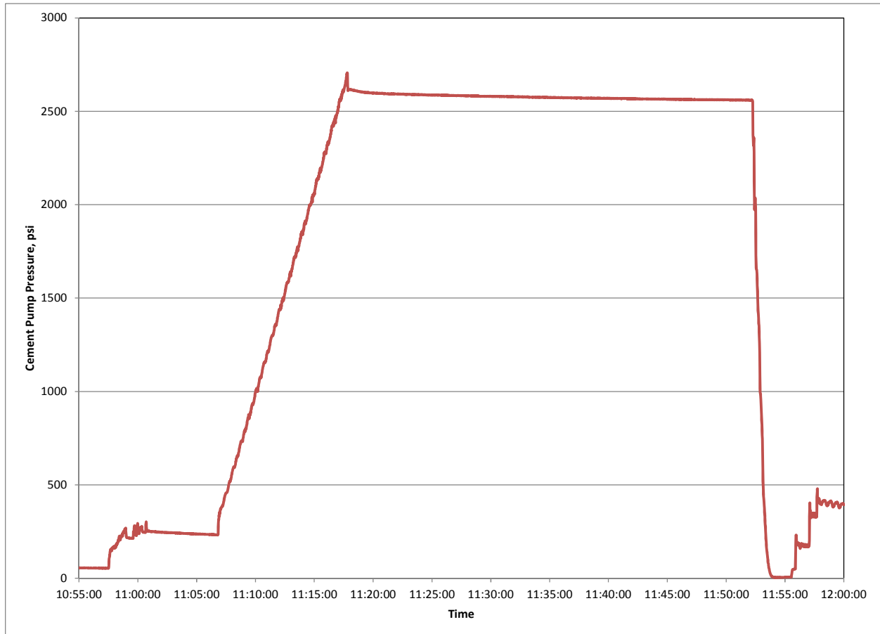
Figure 29: Plot of cement pump pressure recorded during positive pressure test on April 20th
