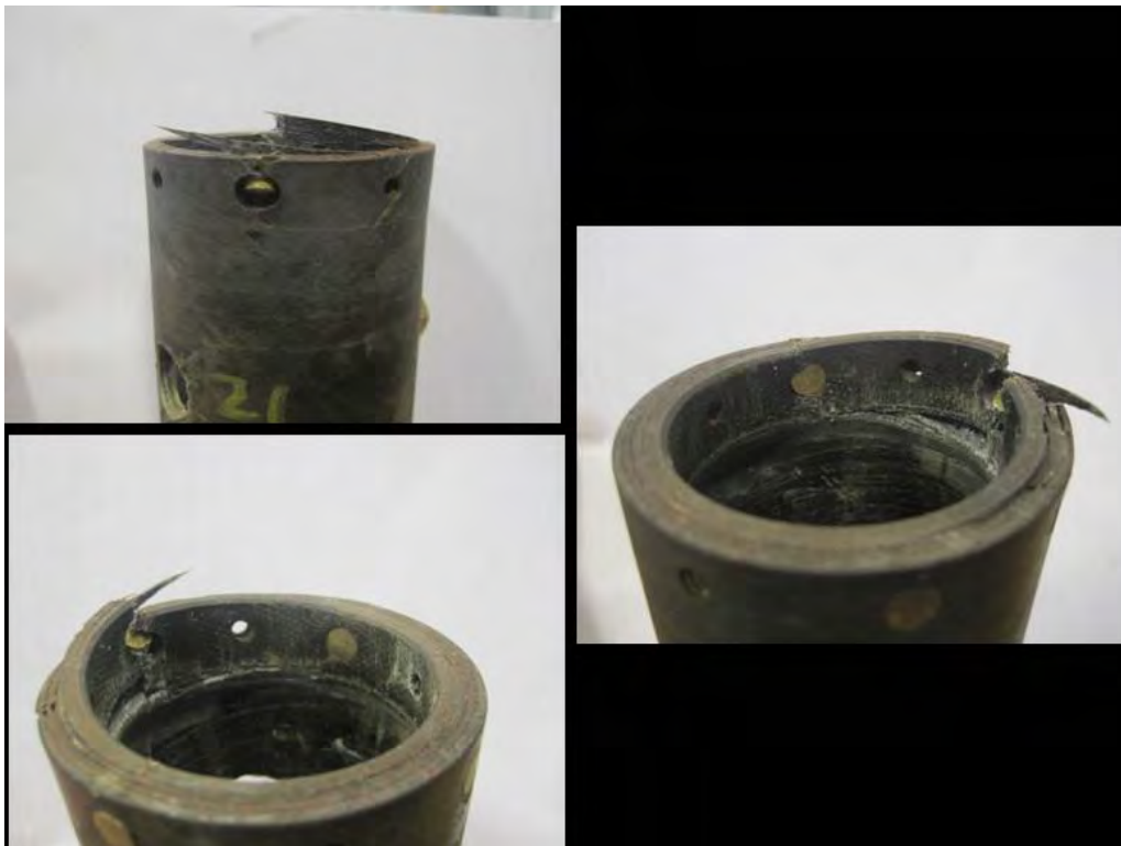
Figure 3.10: Post-test Photographs for Tube Seat Shear Test on Float #2
