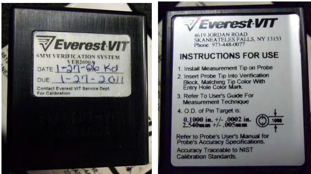
Figure 8: Boroscope Verification Box for Calibration
