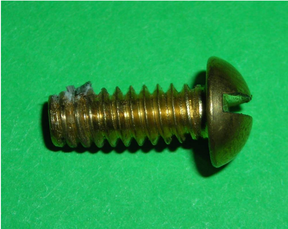
Figure 3.3: Retaining Screw Removed from Float #1 after Conversion Test
