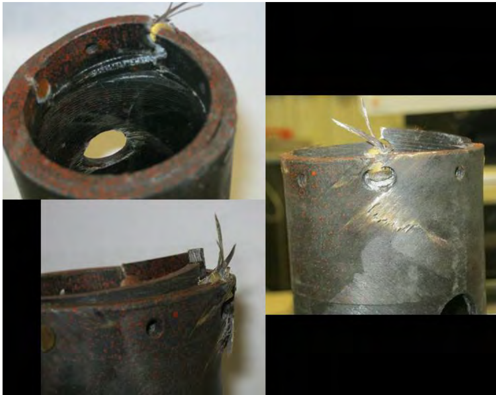
Figure 3.8: Post-test Photographs for Tube Seat Shear Test on Float #1
