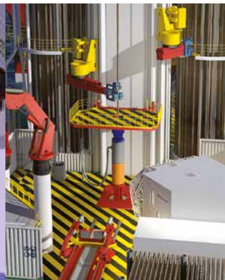
Heave compensated drillfloor
