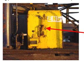
Compound Transmission must be disengaged before shifting the Cotta transmission.
