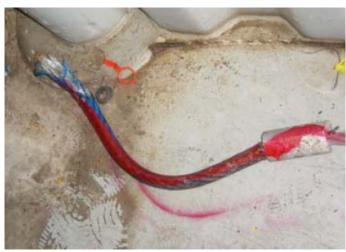
IADC Note: Sling manufacturers recommend that all plastic coating be removed from under the swage before it is crimped. Plastic coating decreases the coefficient of friction required for making a swaged sling.
