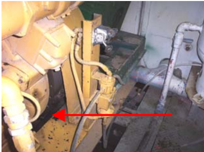
Original clutch assembly guard allowing access to Fly wheel and clutch.
