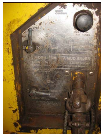
Mud Bucket Control
