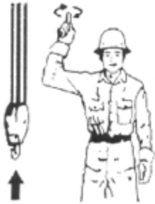
HOIST THE LOAD
