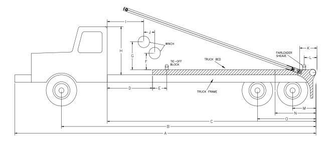
Use the drawing above as a guide and enter the side view measurements indicated in the data table below.
