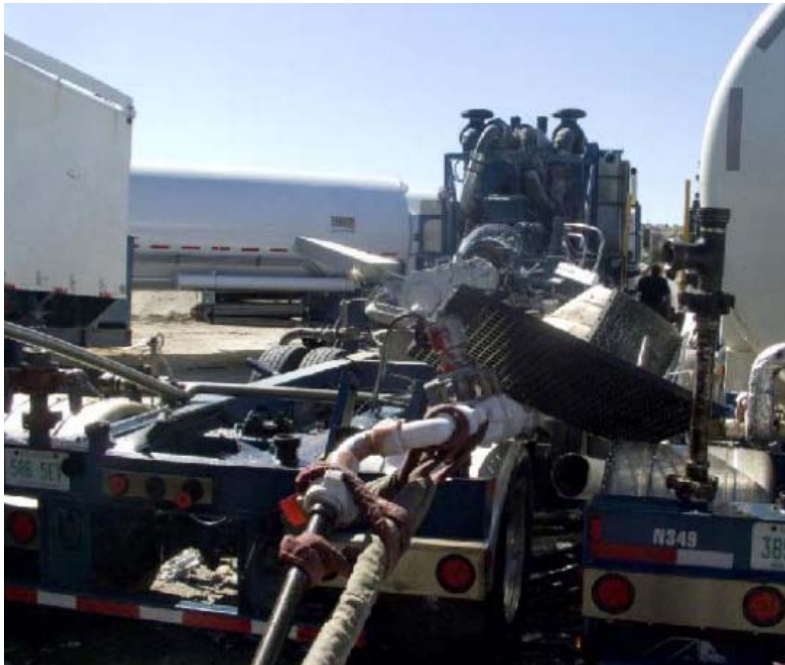
Post Incident – Storage Vessel Missing From Nitrogen Unit
