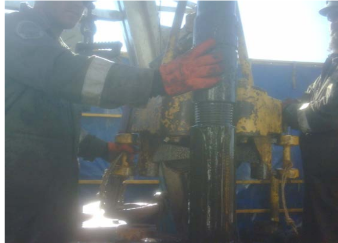
Incorrect Hand Placement
