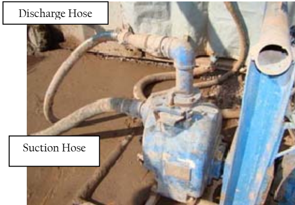
Figure 1 Transfer pump at reserve pit behind mud tanks.
