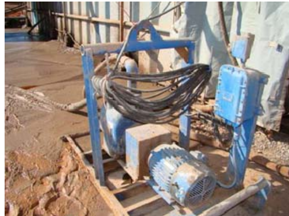
Figure 1 Transfer pump at reserve pit behind mud tanks.
