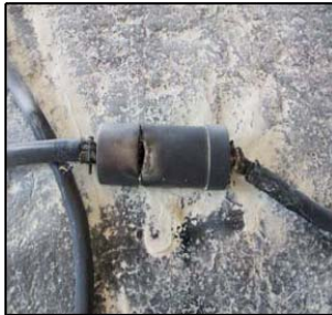
Twist-lock 240-Volt plug & socket after incident.
