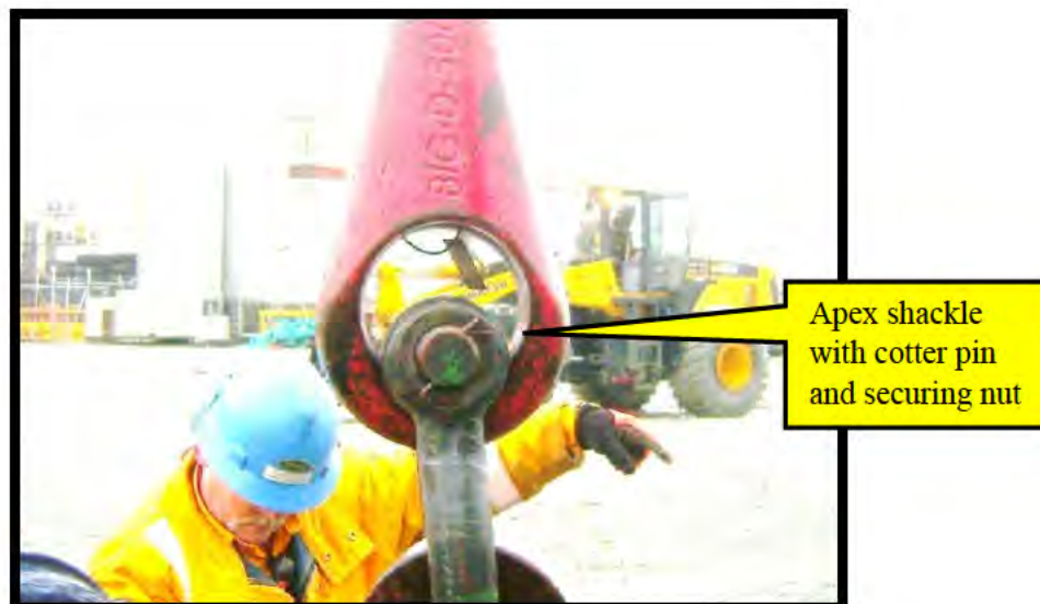
Figure 13: OSI Terminal workers hoist the tow plate and pennant wire. The photo shows the 120 ton shackle (original photo brightness adjusted) with the cotter key. The shackle (described as apex shackle) connects the tow plate to the 100' tow pennant socket. (Photo courtesy of GL Noble Denton, Mr. [REDACTED])
