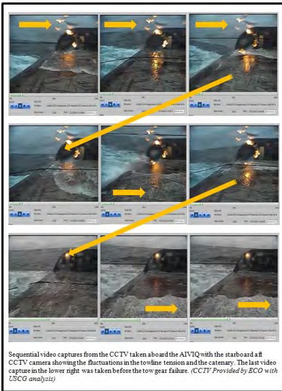
Figure 67 – Movement of AIVIQ towline and tension on the line on the morning of December 27, 2012.
