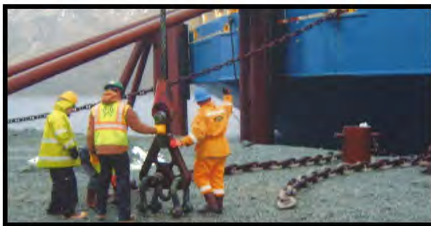
Figure 14: Preparing to Connect the Towing Plate to the Bridle Legs (Photo courtesy of GL Noble Denton, Mr. [REDACTED])
