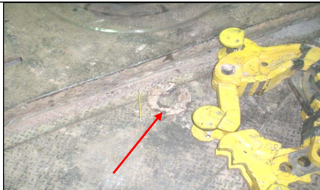
Tong counter weight segment landed beside rotary table and bounced a further 5-6 feet.
