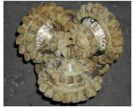
The first new bits, the 11 5/8-in. ETS13, had a successful bearing design but showed dull conditions.
