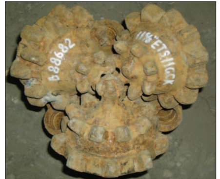
The second series of bits ran to TD with effective bearings in 1 run and drilled at an average ROP of 30 m/hr.
