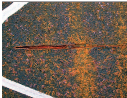
Figures 2 (above) and 3 show that in a second trial run, 2 joints of casing had surface indications, identifying a need for an enhanced pipe inspection.
