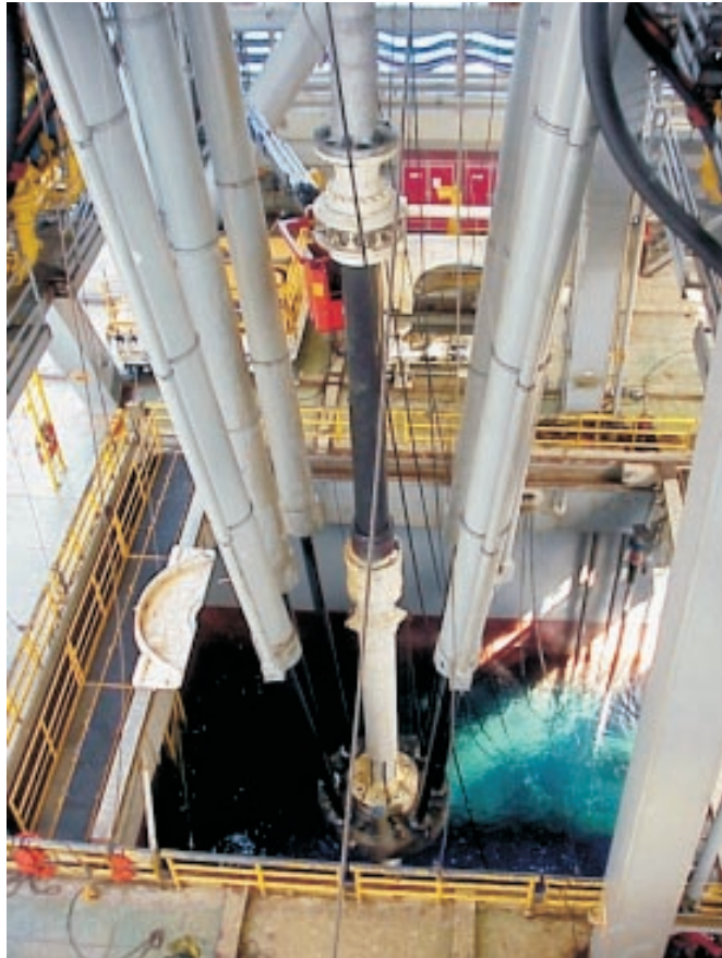
N-Line Drilling Riser Tensioning System increases allowable deck space and reduces weight. It also lowers operating and maintenance costs.
