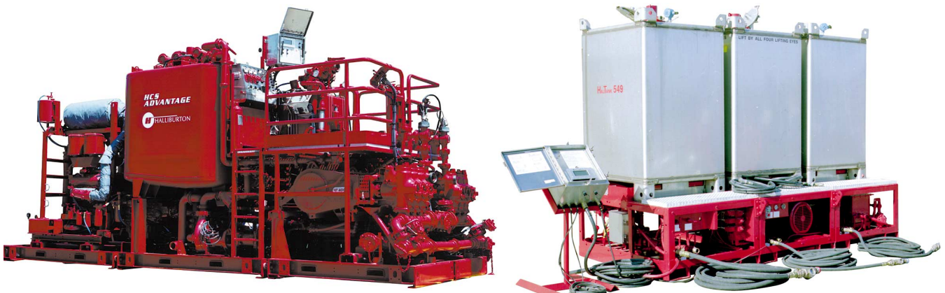
Cementing equipment: Figure 2 (left) shows a cementing skid equipped with recirculating cement mixer (RCM) and automatic density control systems. The RCM has evolved to allow routine mixing of high-density or thixotropic slurries at high through-puts. Figure 3 shows continuous metering system (CMS) liquid-additive tanks. The CMS allows highly accurate injection of additives at various points in the mixing/pumping process.
