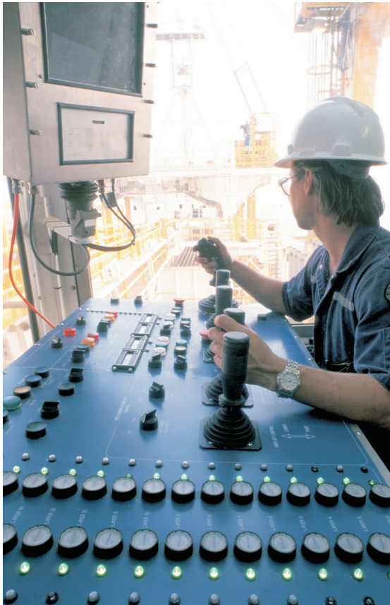
The Assistant Driller aboard GlobalSantaFe's drillship C R Luigs operates the pipe racking machine.
