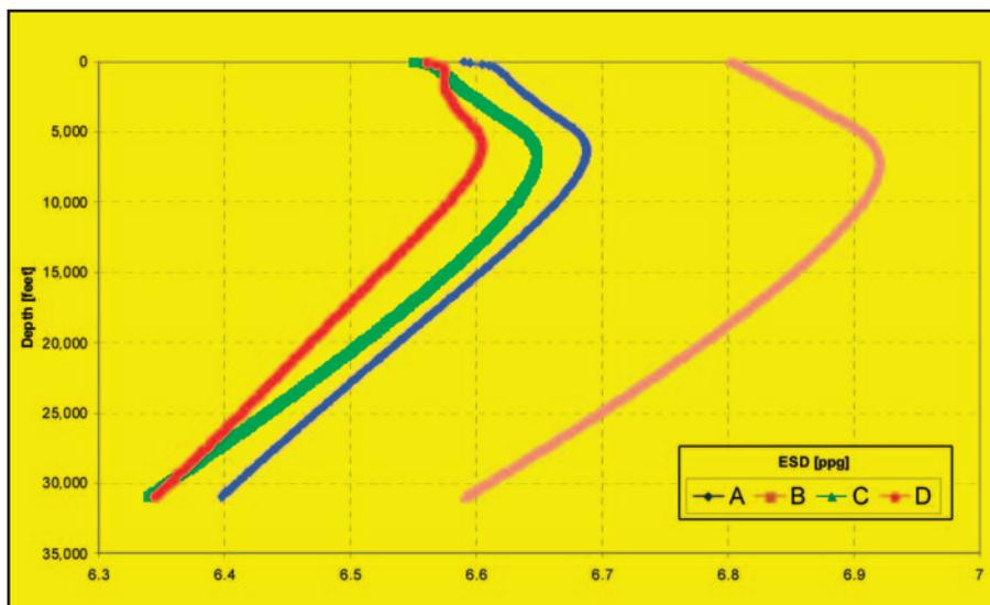
Base-fluid equivalent static density (ESD) comparison of four commonly used base-fluids as a function of depth (at predicted pressures and temperatures).
