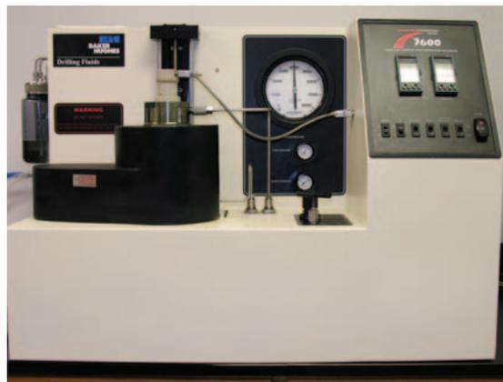
The Chandler 7600 HPHT mud viscometer is designed for 40,000 psig/600°F operating conditions.
