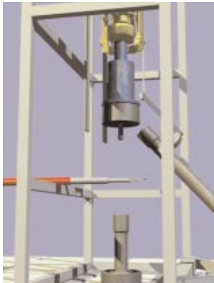
SPE/IADC 52770: This new casing-running tool, developed by QCD, Deutag and their partners, employs the top drive as a torque wrench.
