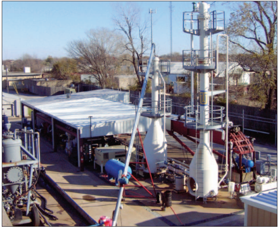
The test facility simulates conventional and UB drilling operations at downhole conditions.
