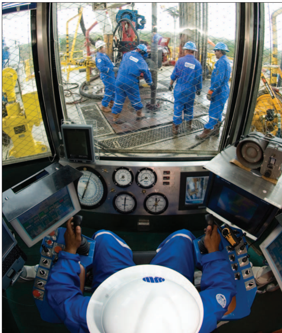
Above, sensors placed around the rig send critical information to the sophisticated drilling console, which controls operations of the rig. Below, a PACE rig, Rig 669, drills for Sincor in Venezuela.
