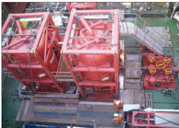
Figure 1: To deal with pressure control and lost circulation problems in the Gullfaks field, operator Statoil decided to pursue a solution that would include a full UBD-compliant, 4-phase separation package using clear brine as drilling fluid.
