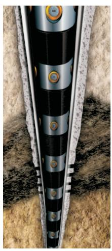
Halliburton's third generation crossed dipole sonic tool makes it easy to determine fast and slow shear wave travel times and their orientation in the formation.
