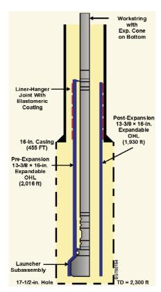
A record length OHL system was installed as an extension of 16-in. conductor casing in S Texas.
