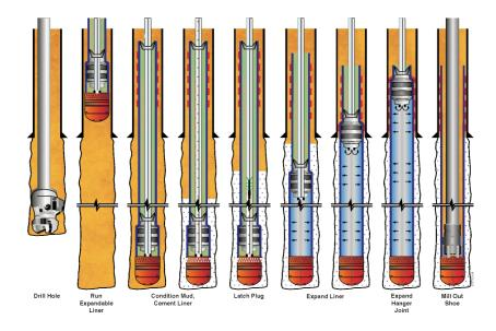
Installation of the Expandable Openhole Liner System involves, from left: Drill hole; run expandable liner; condition mud, cement liner; latch plug; expand liner; expand hanger joint; and mill out shoe.
