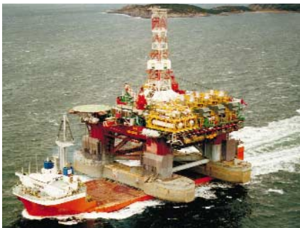
Dockwise's Mighty Servant 1 set a new record in transporting the 32,767-ton semisubmersible Petrobras 36.
