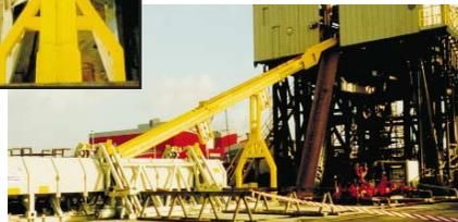
**Mechanized catwalk system: The Bentec-designed mechanized catwalk system aims at simplifying and speeding the transport of drillpipe or casing from pipe rack to drill floor.**
