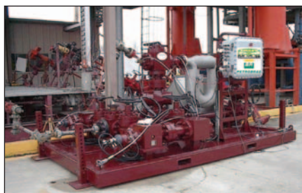
Above, a screen shot shows the basic screen of the system, displaying the flows in and out, mud weights in and out, the pressures, and well as the sketch of the downhole conditions, with the most important values for the driller to better understand what is happening downhole. Below, the Secure Drilling manifold is shown during field tests at Louisiana State University. The tests were conducted between October 2005 and March 2006.
