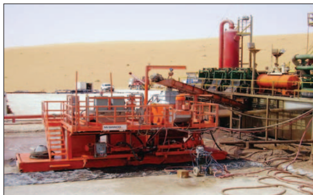
■ The VERTI-G cuttings dryer has been used on more than 147 wells.
