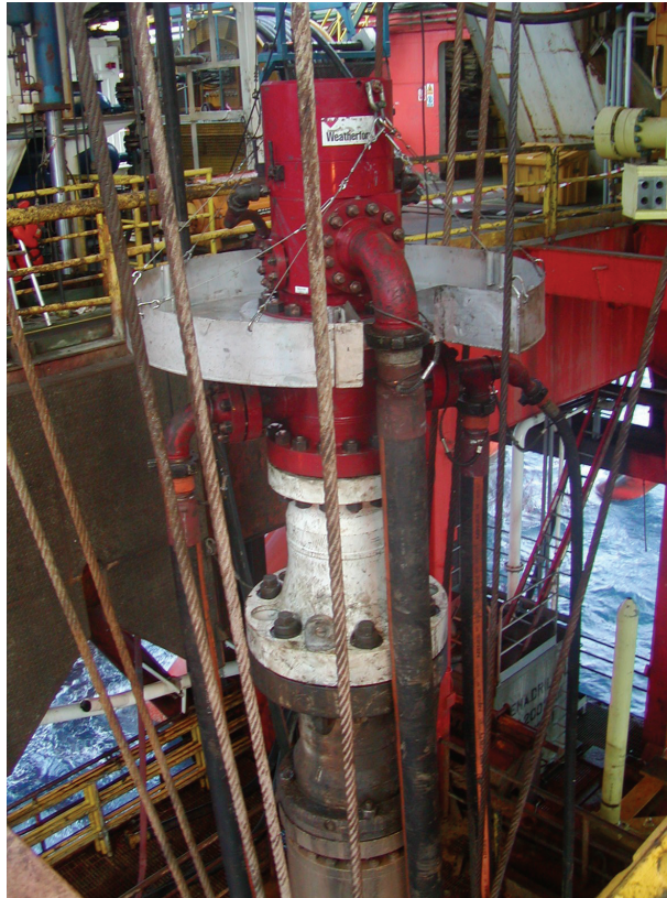
A riser cap is installed on a well in Malaysia in preparation for drilling a well utilizing managed pressure drilling technology.
