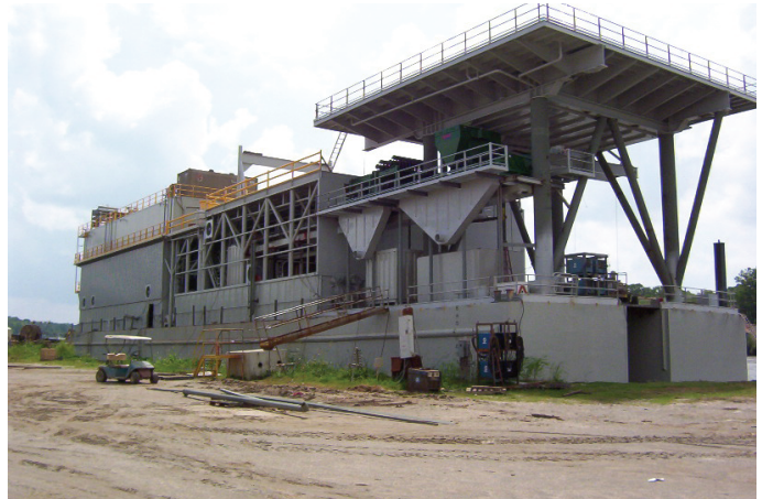
Coastal Drilling Company's newest inland drill barge, Rig 21, is shown here under construction at Semco Shipyard in Lafitte, Louisiana. The rig is scheduled for delivery this summer.
