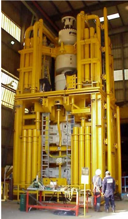
Typical 5-ram with subsea accumulator (DP Rig)
